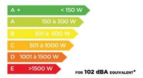
\*The figure given represents the electrical power dissipated by the speaker to generate over its bandwidth a sound level equivalent to 102 dBA with a pink noise input. For calculation purposes, the speaker is considered being part of an equalized sysytem with absolutely flat response from 20 Hz to 20 kHz.
